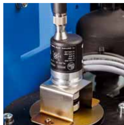
Linear measurement by means of a counter: Rotary movement is converted into digital signals.
