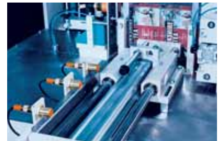
The sensor switches as soon as the magnet has reached the switch-on point. The direction of movement of the magnet is not important.
