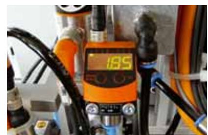
Pressure measurement in pneumatic systems.
