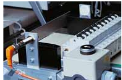
The reflector reflects the light beam: For a retro-reflective sensor transmitter and receiver are integrated into one housing.
